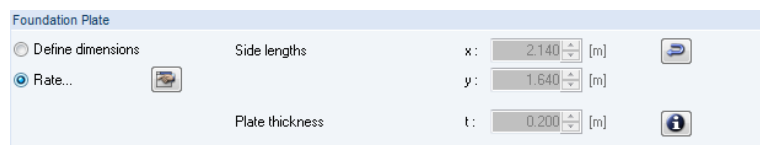
Figure 2.17: Defining or rating the foundation plate dimensions
